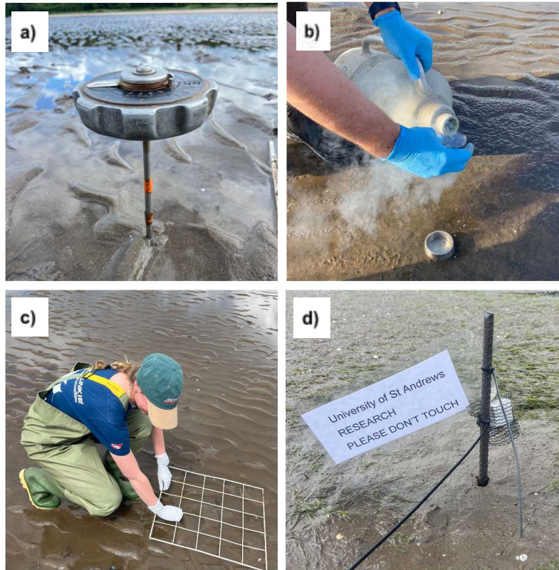
Figure 4. Data collection of a) sediment stability using a shear vane; b) sediment sample using a contact corer; c) worm density using a quadrat; and d) hydrodynamics using the erosion of plaster as a proxy.
